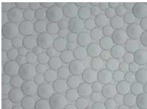
**Fig. 8:** Swollen resin beads under the microscope.
