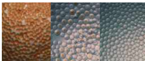
Fig. 4. TNBS-test. Beads inspected under the microscope. left: positive middle: incomplete coupling right: negative.
