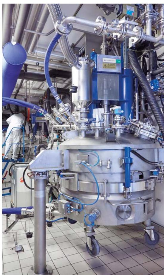
**Stirred-bed technology (SBT) for solid-phase oligonucleotide synthesis (SPOS) represents an economical engineering solution with a relatively simple reactor design. An example of a specific 1000 L stirred-bed reactor Bachem is shown here.**
