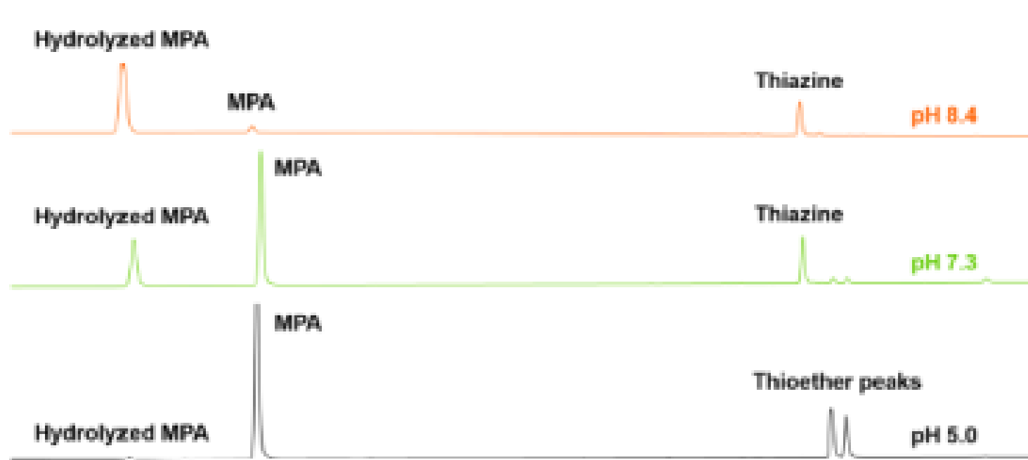
Figure 3 - UHPLC analysis of CGF conjugation to 3-maleimidopropionic acid (MPA) after 24h at pH 5.0 (black), pH 7.3 (green), and pH 8.4 (orange).
